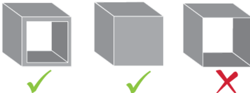
The two objects on the left are printable because they are modeled as complete, solid forms. The object on the right is only comprised of open and unclosed surfaces, image provided by sculpteo.com
