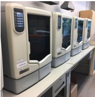
(8 x 6 x 6") and (8 x 8 x 6") ABS plastic, soluble support
